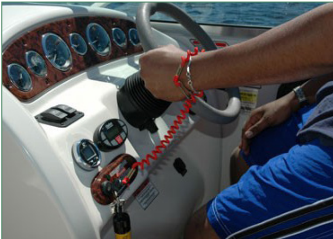
Always use an engine cut-off device to ensure your boat will stop running in the event that you go overboard or are disabled.
